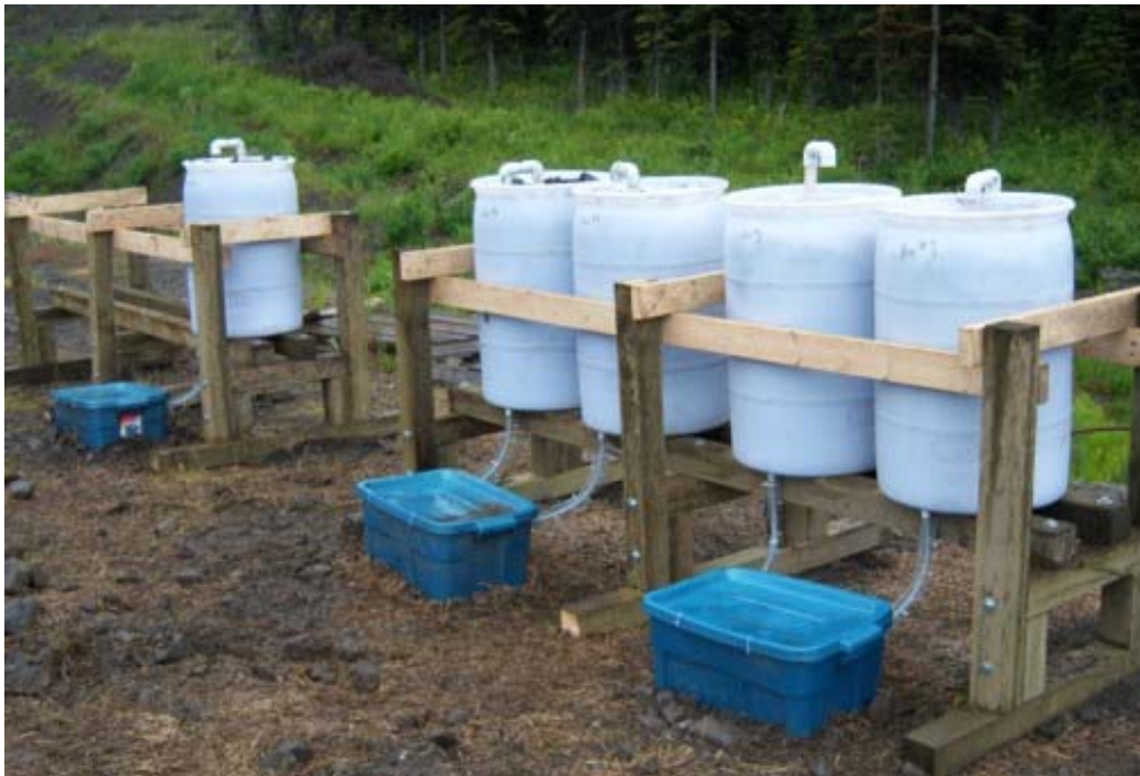
Figure 1: Example of field leach bin experiment set-up.
